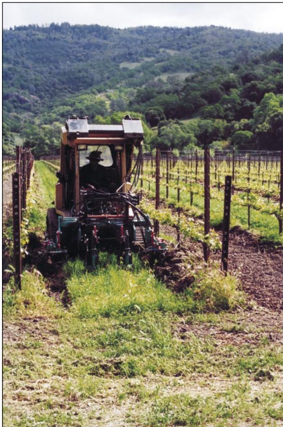
A Clemens Radius vine cultivator is used to remove weeds under vines while leaving between-row cover crops intact.
